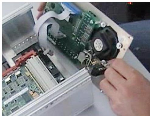
Figure 4, IR44CF II – Remove front panel
