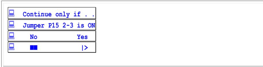
Tab. 16, IR44CF II display – Request for correct setting of jumper P15
