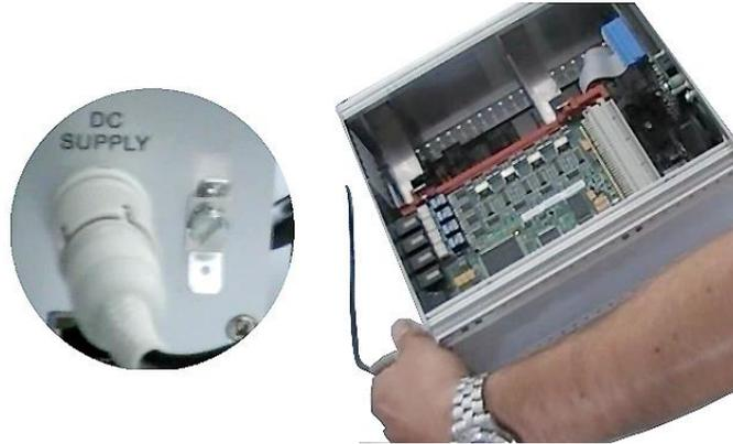
Figure 3, IR44CF II – Remove AC adaptor
