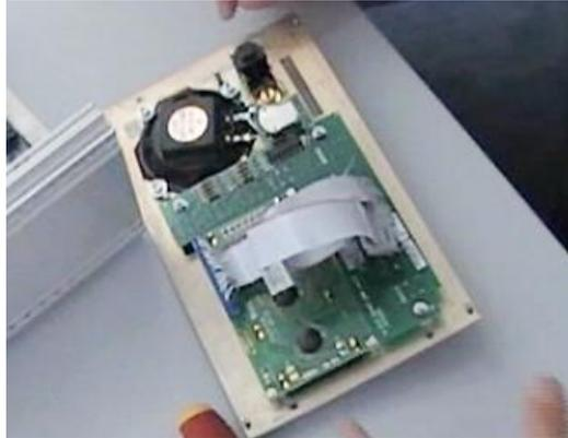
Figure 5, IR44CF II – Front panel removed
