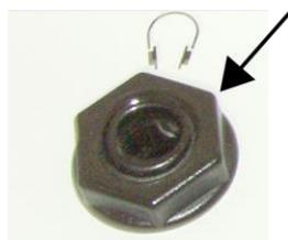
Figure 8, IR44CF II – Headphones output socket mounting nut
