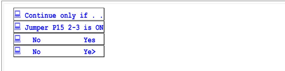
Tab. 36, IR44CF II display – Request for correct setting of jumper P15
