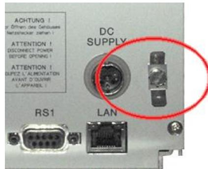
Figure 3, IR44CF II – Ground connection of IR44CF II housing
